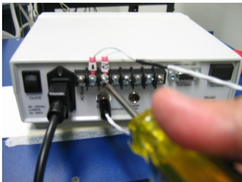
Figure 15, External TEC Controller Connection
