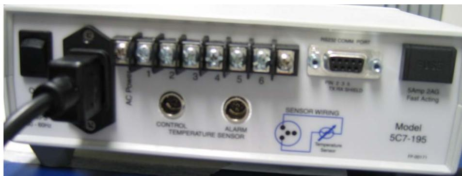
Figure 12, TEC controller Rear Panel
