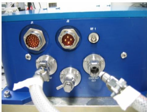
Figure 7, Laser Head Coolant Lines
