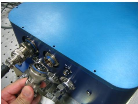
Figure 9, Laser Head Power Connection
