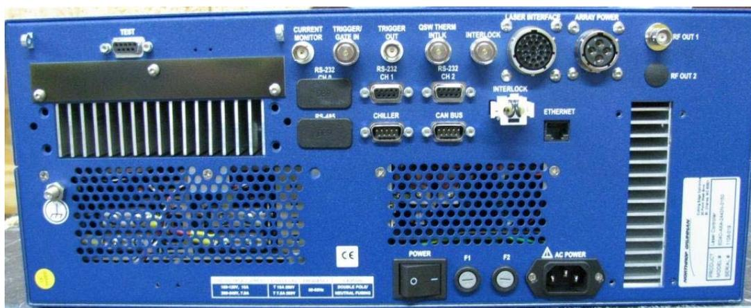
Figure 13, eDrive Rear Panel with Internal TEC Controller (RS232 and RS485 connectors removed)
