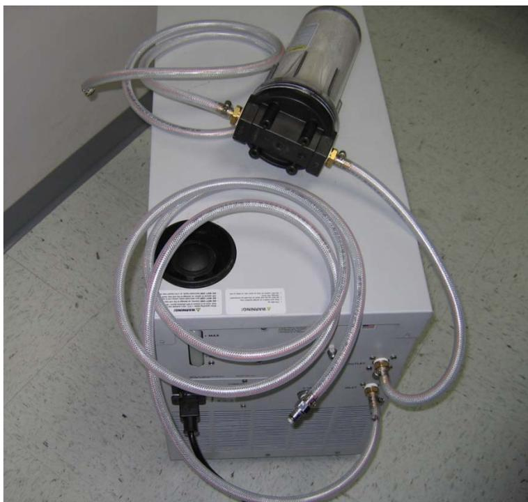
Figure 5, Picture of assembled water hoses, filter with the chiller.
