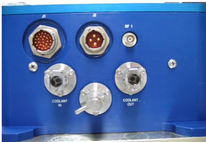
Figure 6, Connectors on the back panel of the Patara laser.
