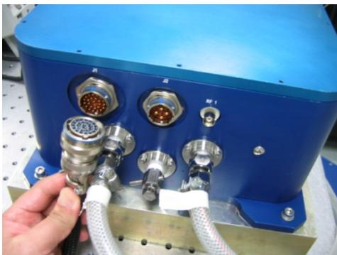
Figure 8, Laser Head Signal Connection
