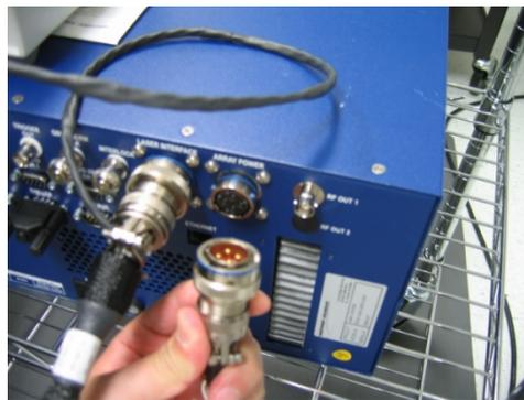
Figure 16, eDrive Array Power Connection
