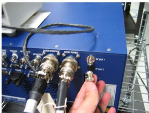
Figure 17, eDrive RF Connection
